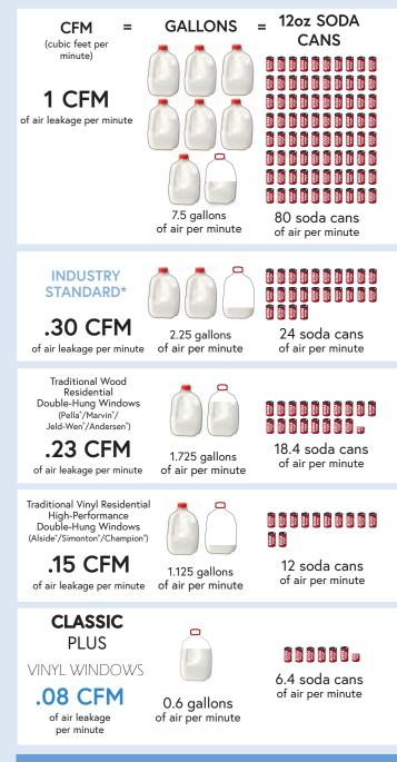
\*INDUSTRY STANDARD: AAMA® (American Architectural Manufacturers Association®) has set the industry standard for maximum allowable air infiltration at 0.30 CFM (cubic feet per minute) during a 25 MPH wind. This is equal to 2.25 gallons or 24 soda cans of air leaking through the window every minute!
